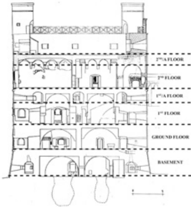
Fig. 5: The south-northern section of the tower with the levels (Feld, Szekér 1994, 178).
