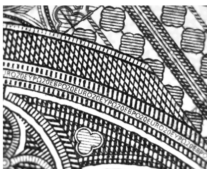
Figure 21. Intaglio: (20 Euro banknote) feathering, relief, Orlof, positive micro-text
