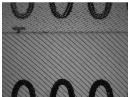
Figure 36. Letterpress — forged example (inkjet V/S letterpress and offset); Dino-Lite microscope image
