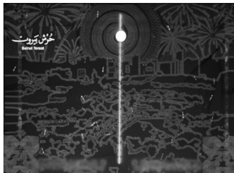
Figure 5. Lebanese biometric passport — invisible fluorescent ultraviolet ink, rainbow printing/IRIS
