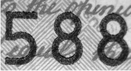
Figure 31. Letterpress — beaded edges, printing interruptions
