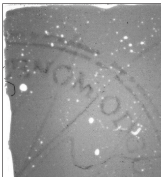
Picture 4.2. The visualization of the transformed into positive: the empty parts of the unreflected lines of the printed letters intersect the reflected signature lines and the stamp print
