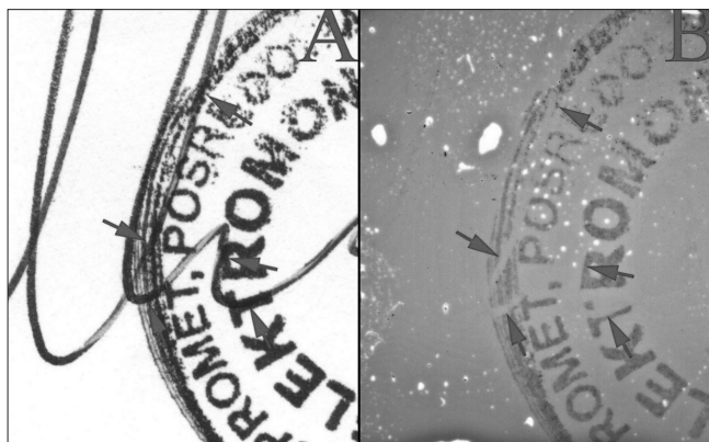
Picture 2.2. The intersection of a signature line and a stamp print in a document (A) and the visualization of the print on the foil transformed into positive (B): there are empty spaces in the stamp mark, which stand in place of unreflected lines made with a ballpoint pen, which intersect the reflected lines of the circles and the letters of the stamp mark
