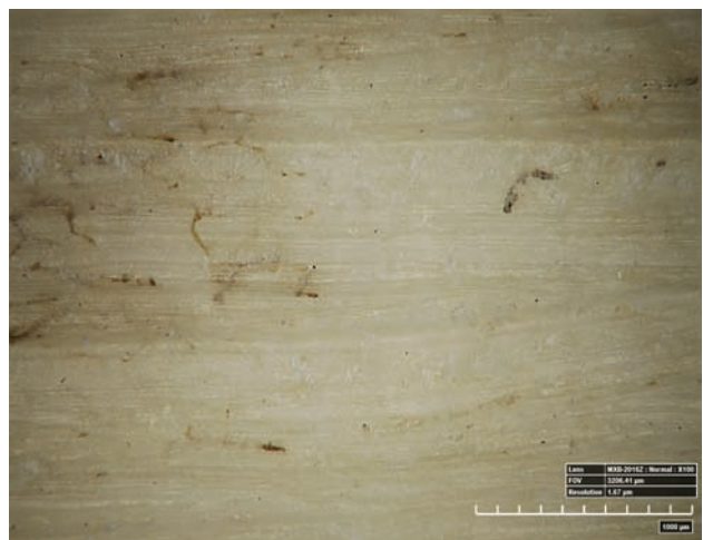
Fig. 17. Experiment. The surface scraped with a worn tool edge. (Photo M. Diakowski)
